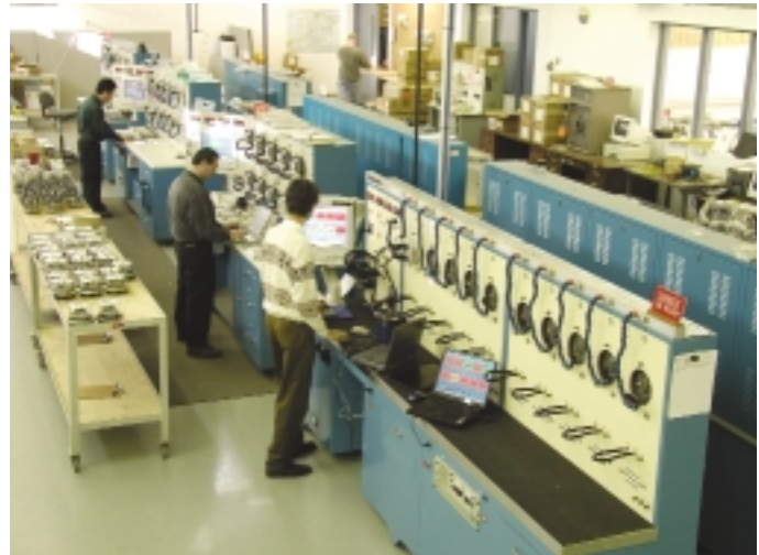
Performing daily accuracy checks and meter verification with Testcor built equipment at Olameter Inc.
